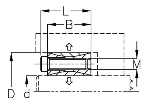
$\begin{array}{lll} {\rm B} \ {\rm mm} & = 20 \\ {\rm d} \ {\rm H8} \ {\rm mm} & = 3865 \\ {\rm D} \ {\rm mm} & = 65 \\ {\rm Fit} \ {\rm tolerance} & = {\rm Aksel} \ {\rm k11-h11}, \ {\rm Nav} \ {\rm N11-H11} \\ {\rm F} \ {\rm kN} \ {\rm torque} & = 58.0 \end{array}$
